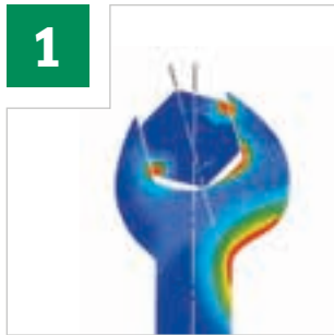
Load zones in standard-quality spanners
