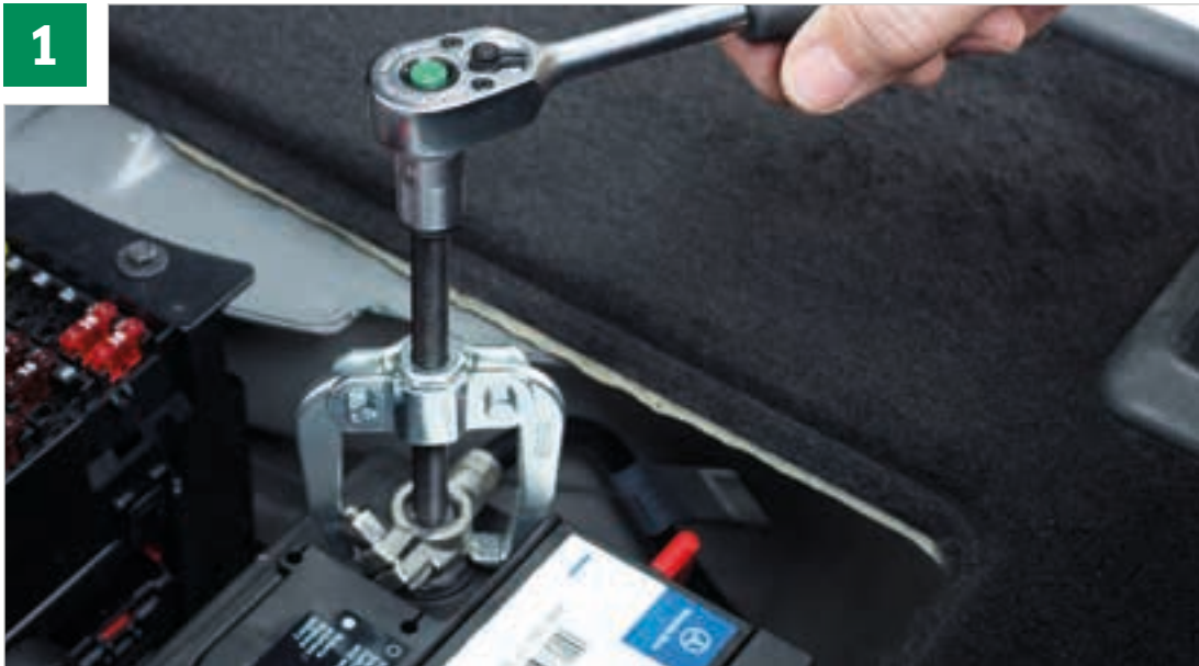
Battery terminal puller in use on a car battery
